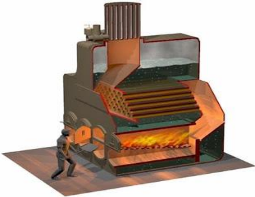
Gambar 8.2 Ketel Uap Pipa Api 1 Pass (1 Laluan)
